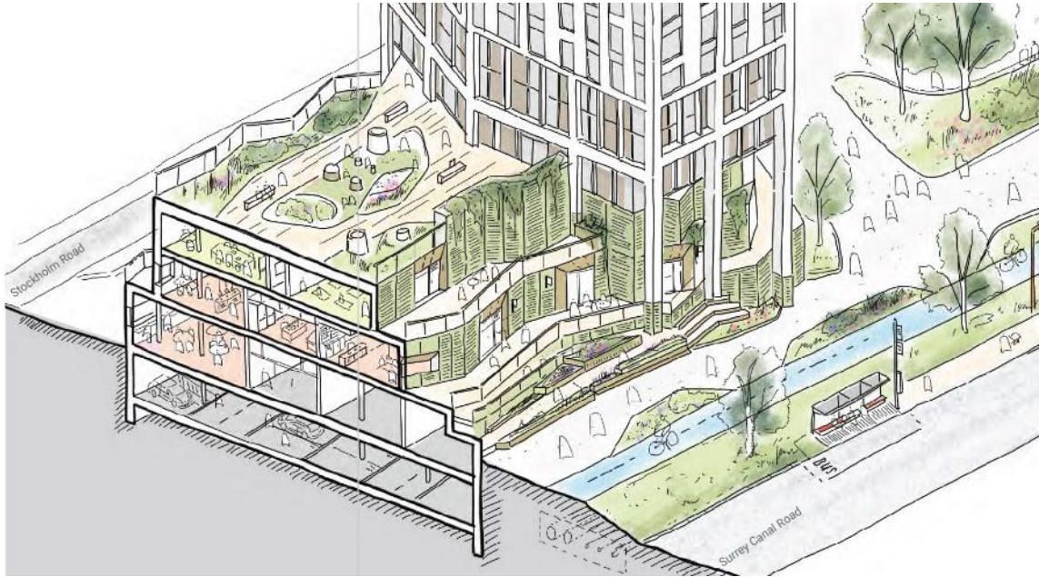
Figure 18 – illustrative sketch diagram showing the approach to stepped and layered podia
